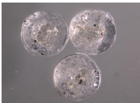
Three samples extracted from three separate polished thin sections. Each core is ~2mm in diameter with the area of interest in the centre. In this example, the olivine crystals contain rare melt inclusions and are being prepared for  $\delta^{11}\text{B}$  isotopic analysis.
