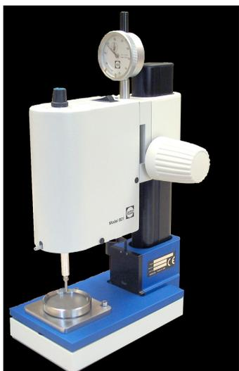
An ultrasonic disk drill is a proven method for producing thin disc shaped specimens from hard, brittle materials such as ceramics, glasses, polished thin sections, and geological materials. This technique produces disks (ID of ~1-3 mm) or cylindrical rods from bulk samples, or cut small diameter holes in thin sections free from significant edge and surface damage.
