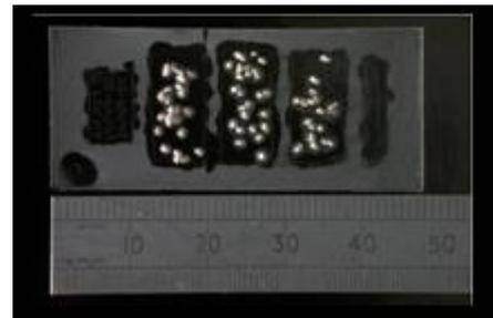
Repeat for other samples until the slide is full. Try to leave a gap between the blocks to prevent cross contamination. Also, be sure to leave a gap of ~4 mm at the top and bottom of the slide - this is important for correct (level) mounting in the e-probe sample holder
